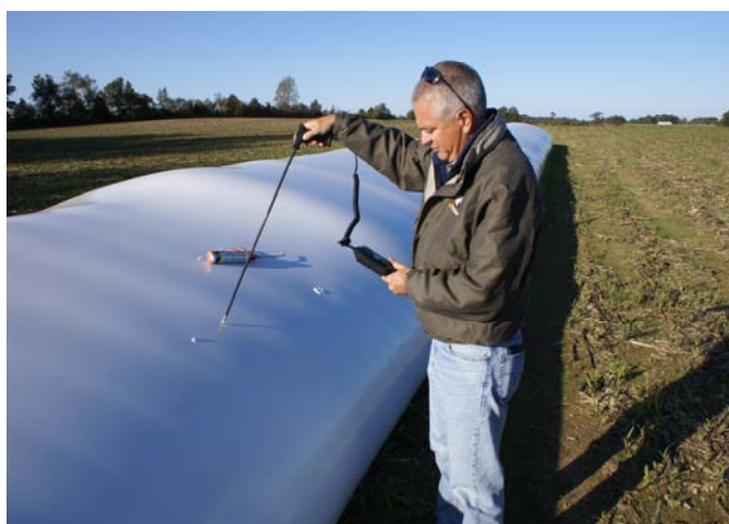
Checking for temperature and moisture using a grain probe
